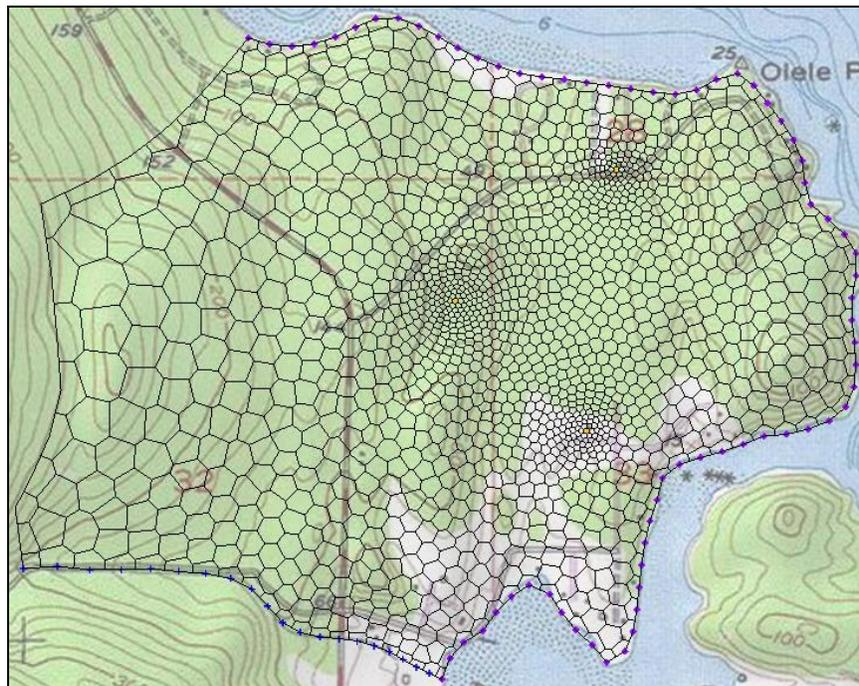
Figure 14 MODFLOW boundary conditions on a Voronoi UGrid
