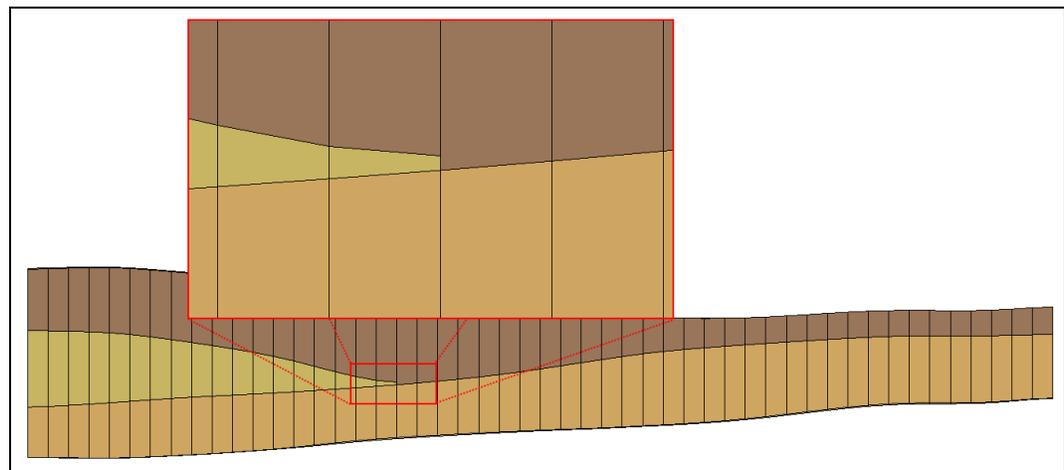
Figure 3 Example of a UGrid with pinching layer
