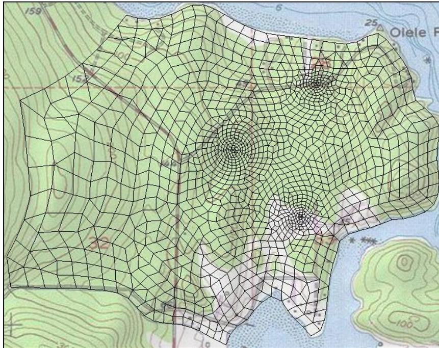
Figure 16 UGrid comprising triangle and quadrilateral cells
