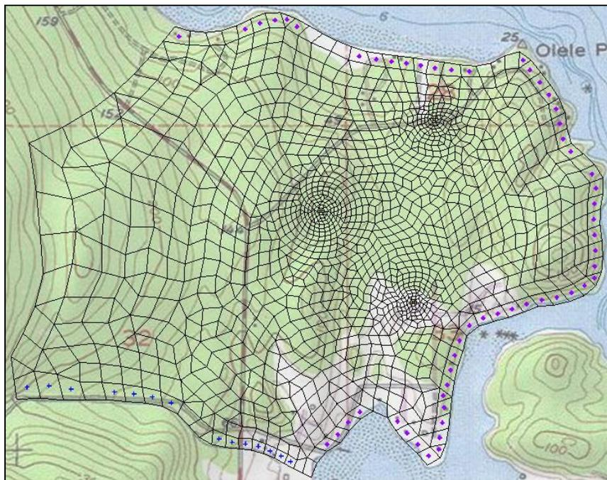
Figure 18 MODFLOW boundary conditions on a 3D UGrid
