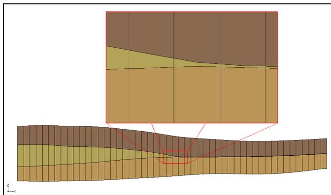
Figure 1 MODFLOW 2000 finite difference grid with pinching layer
