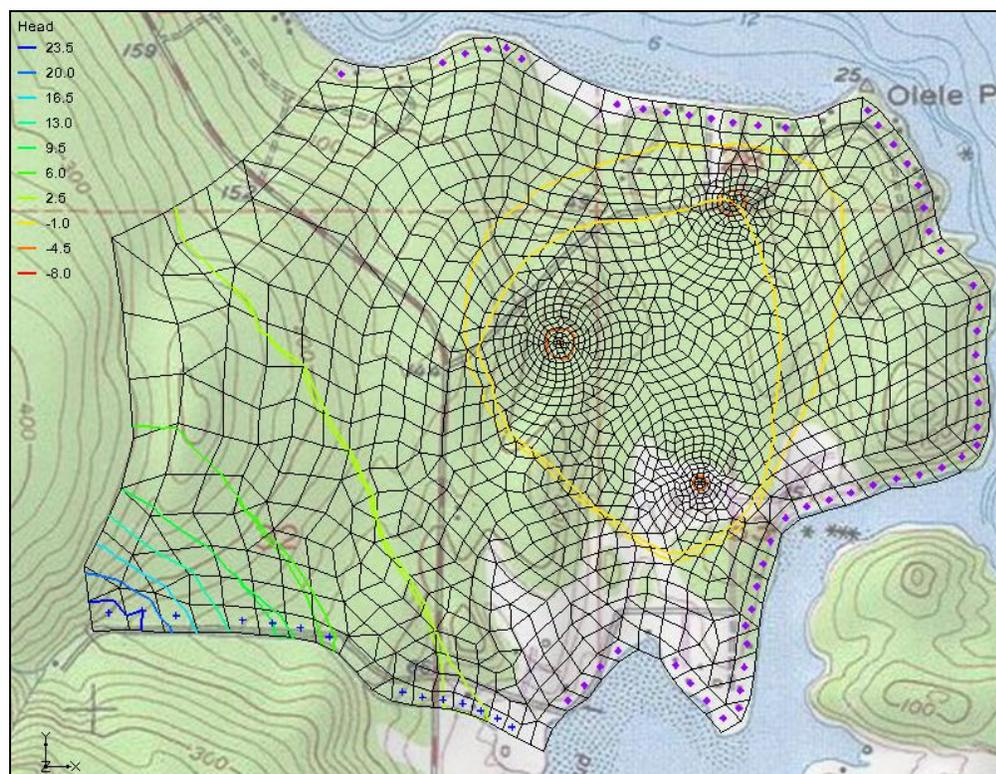
Figure 19 MODFLOW computed head contours on 3D UGrid
