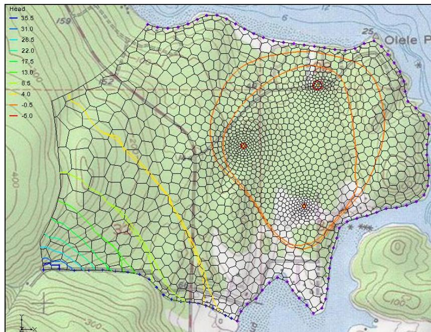
Figure 15 MODFLOW computed head contours on Voronoi UGrid
