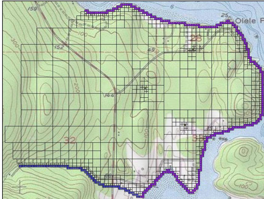
Figure 10 Quadtree UGrid with MODFLOW boundary conditions
