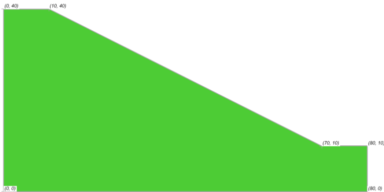
Figure 47 Geometry of the Baker Simple Slope model
