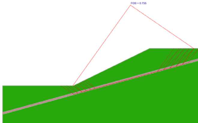
Figure 30 Solution using the Spencer Method
